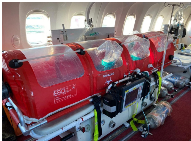
Fig. 1. Patient isolation transport unit (PITU)
